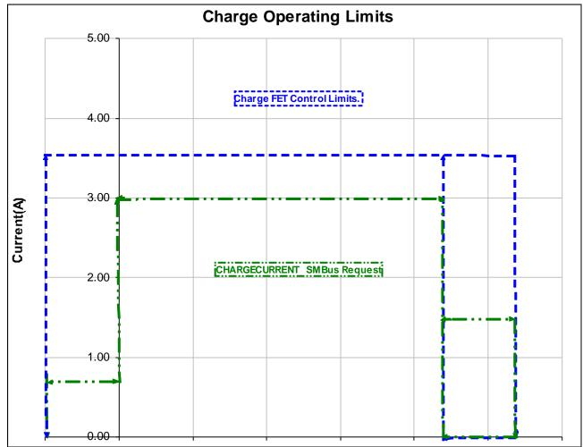
NOTE: If not charging & temperature > 45C then the battery enters Charge-Inhibit where ChargingCurrent() = 0 until temperature  $\le 44C$ .
