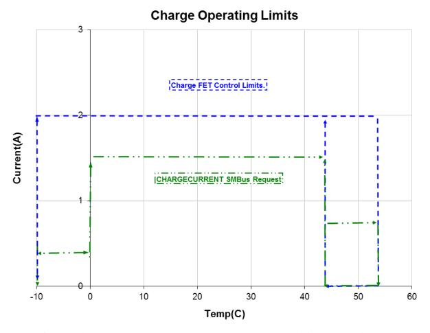
NOTE: If not charging & temperature > 45C then the battery enters Charge-Inhibit where ChargingCurrent() = 0 until temperature <= 44C.
