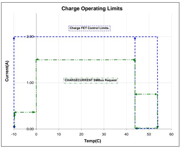
NOTE: If not charging & temperature > 45C then the battery enters Charge-Inhibit where ChargingCurrent() = 0 until temperature <= 44C.
